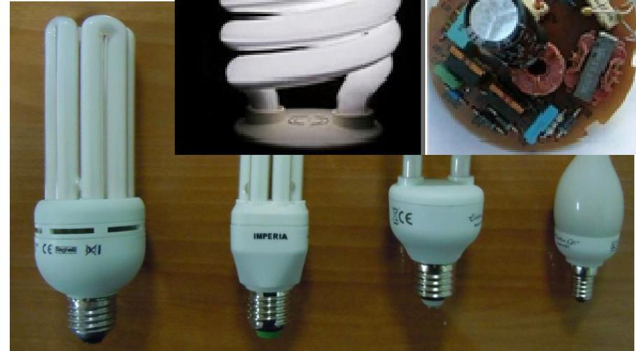
**Due to the high frequency solid state electronic circuitry used in the ballast, CFLs emit a relatively strong electromagnetic field**
