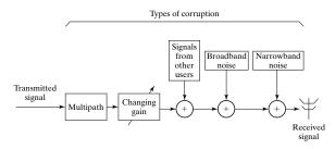
Filtering of the received signal by an appropriate linear system will offer compensation in each case.
