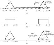
The Signal-to-Noise Ratio (SNR) is the ratio of the power of the signal (the area under the triangles) to the power in the noise (the shaded area). After BPF of sum, noise  $\downarrow$  and SNR  $\uparrow$ .
