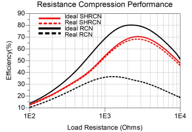
Fig. 7. Comparison of resistance compression performance between SHRCN-based rectifier and conventional RCN-based rectifier at input power of -2dBm.
