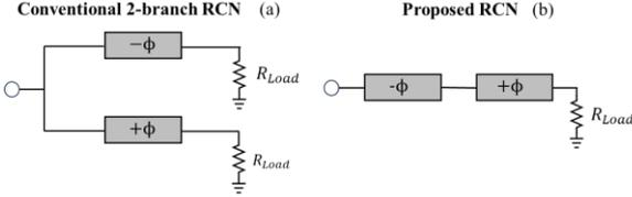
Fig. 2. (a) Conventional two-branch rectifier vs. (b) proposed SHRCT.
