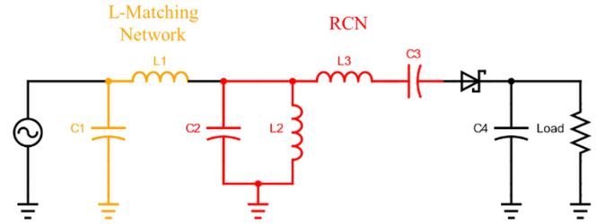
Fig. 6. A lumped-element-based rectifier optimized using conventional RCN and L-matching network.
