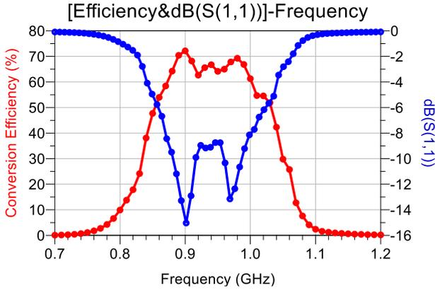
Fig. 3. Simulated conversion efficiency and  $S_{11}$  versus operating frequency at input power of 0 dBm and load resistance of 2 k $\Omega$ .
