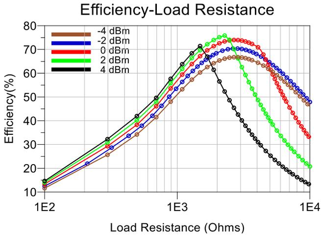
Fig. 4. Resistance compression performance of the SHRCN-based rectifier for various input power levels ( $P_{in} = -4, -2, 0, 2, \text{ and } 4$  dBm) at 900 MHz.
