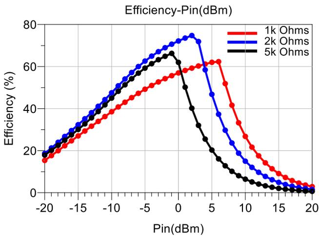
Fig. 5. Conversion efficiency versus input power levels for load resistance  $R_L = 1000, 2000, \text{ and } 5000 \Omega$  at 900 MHz.
