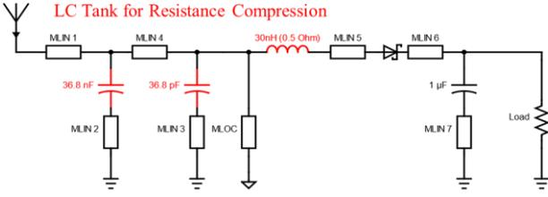
Fig. 1. Detailed schematic of the proposed single-branch resistance compression circuit topology together with the rectifier.
