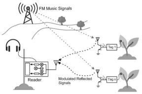
Figure 1. Backscatter communication using ambient Frequency Modulated (FM) signals. A commecrial FM receiver can be used for collecting the data.
